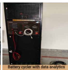
Battery cycler with data analytics
