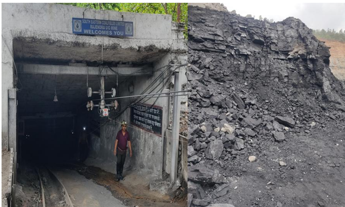
Figure 2.9 Field photograph showing an Incline (passage connecting to the underground coal reserve) of an underground mine and open caste mine from where the samples have been collected.
