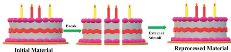
Figure 1.2: Reprocessable property of dynamic covalent networks.
