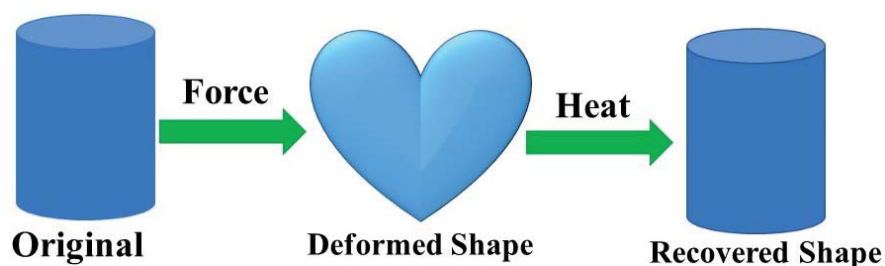
Figure 1.3: Shape memory performance of dynamic covalent networks.
