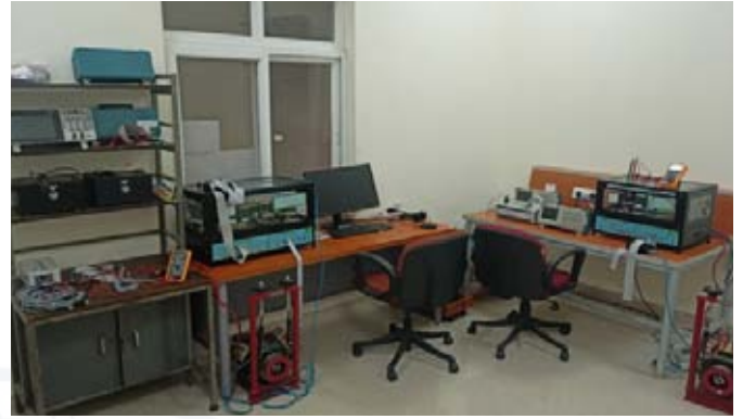
Multiphase (5-phase and 9-phase) Motor Drives (Hardware setup for real time implementation)
