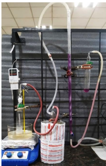
Figure 2.9 The set-up made for the measurement of generated H 2 gas in the reaction.
