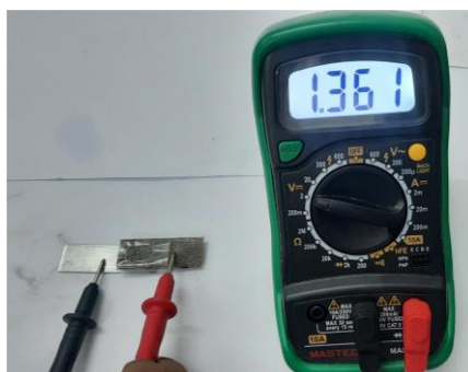
Figure 5.36 Photograph displaying measured open-circuit voltage of ~1.361 V using PAM-h electrolyte for NiO/Ni-SACs/mNC1000.
