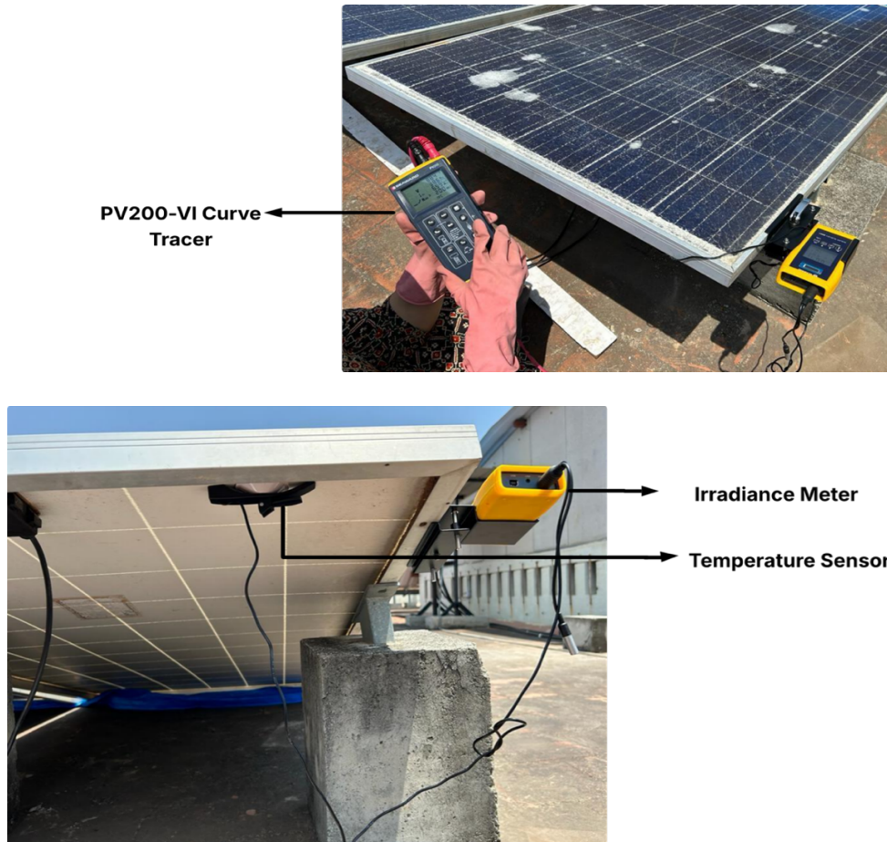
Fig 4.7. VI Curve tracer coupled with irradiance meter and temperature sensor for the considered system
