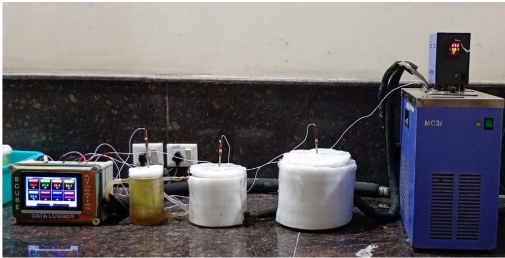
Figure 4.5 : Experimental Setup for 600 ml, 2 L and 5 L reactors connected in series
